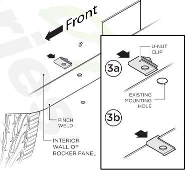
4. On passenger side of vehicle, align Front, Center and Rear Brackets as shown.
