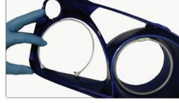
C) Use adhesive to hold the ring in place on the housing. Make sure you give it time to set before begining the next step.
