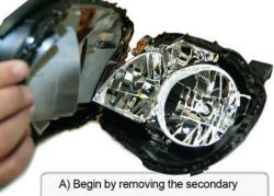
A) Begin by removing the secondary housing from the main assembly. This is where the rings will be placed.
