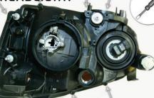
C) If the lens does not separate re-heat the light for 5 minutes and try again
