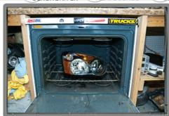
STEP # I: IN ORDER TO OPEN THE LIGHT WE WILL FIRST NEED TO HEAT THE HOUSING. IF USING A HEAT GUN BEGIN BY HEATING THE SEAL EVENLY WHILE CONSTANTLY MOVING THE HEAT GUN. IF USING AN OVEN: PREHEAT TO 225°F AND PLACE THE LIGHT IN THE OVEN FOR IO MINUTES.
