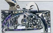
Again, drill another small hole into the chrome housing. Be precise with drilling. You do not want to scratch the chrome surface.
