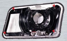
Remove these four T-10 Torx Screws first.
