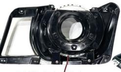
Re-install the Bezel and tighten down the four T-10 Torx Screws
