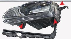
Start by using a phillips screwdriver to remove this bracket. There are 3 screws holding it in place.
