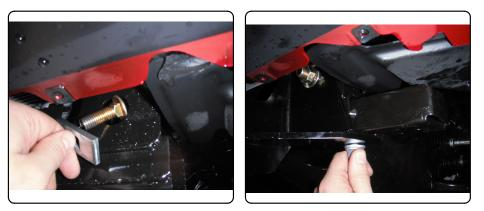
4. Torque all 12mm fasteners to 86 lb-ft and all 1/2" fasteners to 110 ft-lb.
