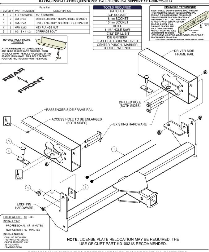
PERIODICALLY CHECK THIS RECEIVER HITCH TO ENSURE THAT ALL FASTENERS ARE TIGHT AND THAT ALL STRUCTURAL COMPONENTS ARE SOUND.
