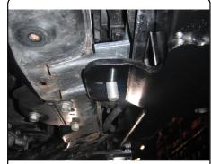
8. Fishwire the top 7/16-14 x 1-1/4" bolt through hitch and side plates and install 7/16-14 hex flange nuts.
