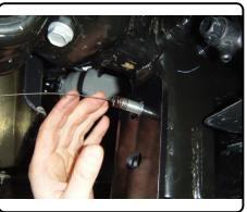
6. Torque all M12 hardware to 79 ft-lbs and 7/16 in hardware to 70 ft-lbs.
