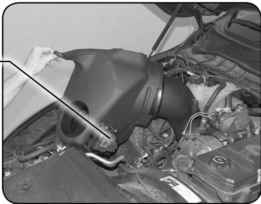
**STEP 21** - Insert the Jammer housing down into the engine compartment pushing the pins on the bottom of the housing into the rubber grommets on the fender well. Ensure the pins are engaged into the grommets by making sure the housing is held in position and is not easily removed.
