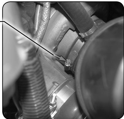
**STEP 7** - The factory Ram Active Air® actuator and door must be removed from the stock air housing and installed in the Jammer housing.
