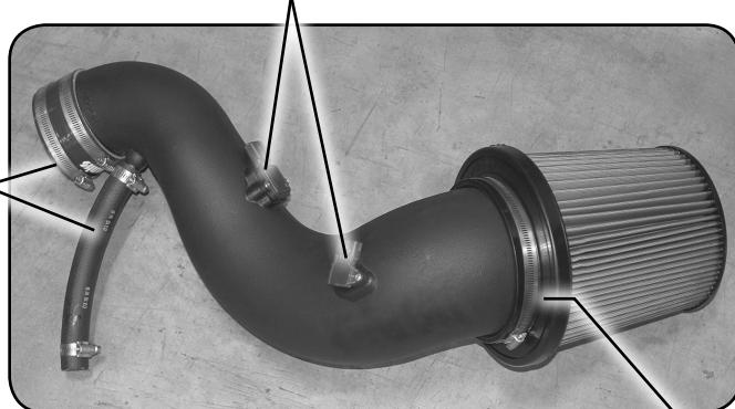
**STEP 16** - Install the Jammer Filter onto the Intake Tube and secure with the hose clamp. The hose clamp must be held up against the base of the filter while tightening the clamp.
