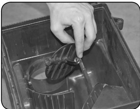
**STEP 12** - Install the Ram Active Air® door and actuator motor into the Jammer housing. Begin to insert the actuator motor from the side and hold the door inside the housing. Slide the door over the actuator motor shaft. Make sure the door and actuator motor are oriented correctly. When the door is fully inserted over the shaft you will feel a click and the door will not pull from the shaft easily.
