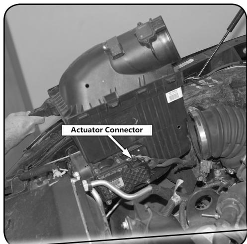
**STEP 6** - Loosen the hose clamp holding the intake tube to the compressor inlet and remove the intake tube from the vehicle.
