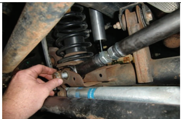
Short end gets straight zerk, long end gets 90 degree zerk
