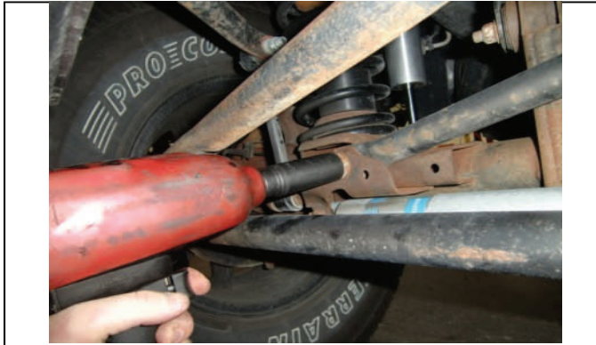
With vehicle on level ground, remove track bar bolt at axle
