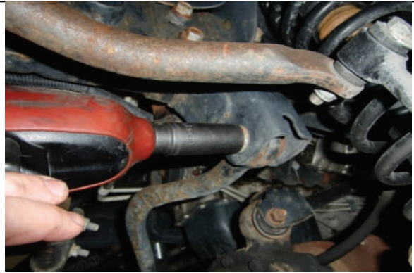
Remove hardware at the frame as well.
