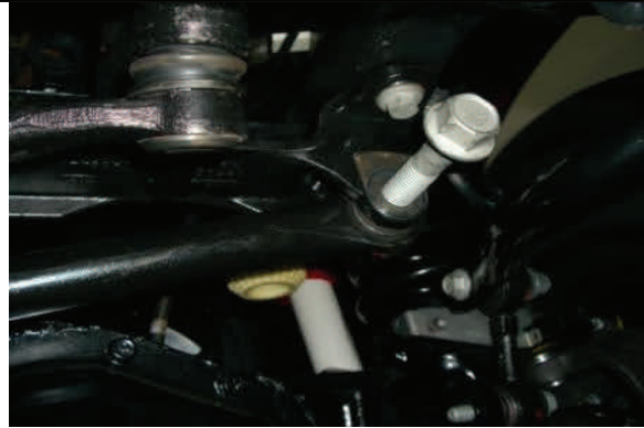
Remove upper trac bar hardware at frame
