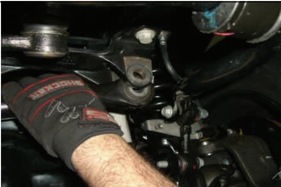
Pull down trac bar or use pry bar to disconnect
