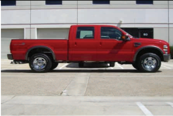
Position vehicle on level ground with steering wheel straight
