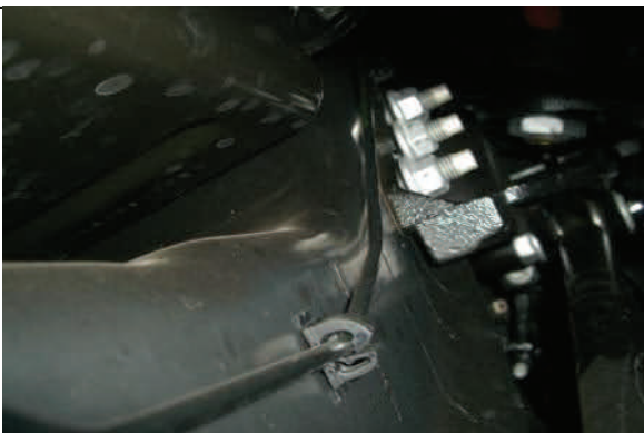
Remove (3) mounting nuts on cross member
