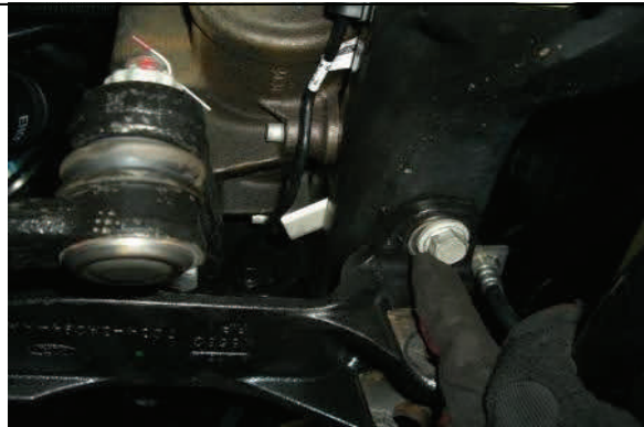
Remove (2) mounting bolts at frame
