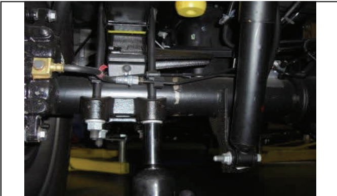
Remove U-bolt nuts and axle mounting plate.
