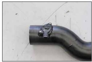
16. Install the mass air sensor into the K&N $^{\! @}$  intake tube and secure with the provided hardware.
