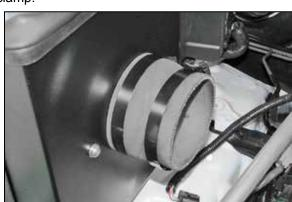
14. Install the provided step coupler (08496) onto the filter adapter and secure with the provided hose clamp.
