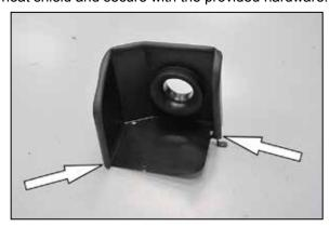
11. Install the provided edge trim onto the  $K\&N^{\otimes}$  heat shield as shown.
