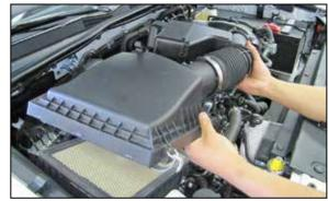
6. Release the two clips securing the air filter housing and then remove the intake tube and air filter hosing along with the factory air filter.
