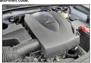
2. Lift up the engine cover to dislodge it from the mounting studs and then remove it from the vehicle.
