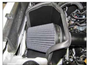
21. Install the  $K\&N^{\otimes}$  air filter onto the filter adapter and secure with the provided hose clamp.
