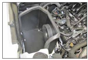
12. Install the heat shield onto the rubber mounted studs installed in the earlier step and secure with the provided hardware.
