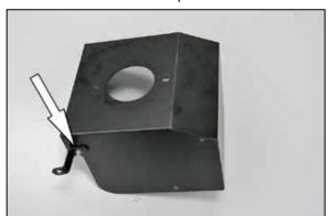
9. Install the provided heat shield bracket (07958) onto the K&N® heat shield as shown.
