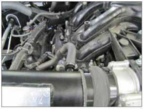
19. Connect the crank case vent fitting onto the vent fitting installed into the K&N® intake tube.
