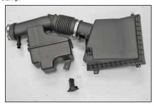
15. Remove the mass air sensor from the factory air filter housing.
