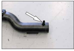
17. Install the provided NPT vent fitting into the K&N® intake tube as shown.
