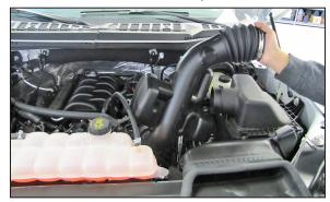
4. Unhook the coolant line from the intake tube and then remove the intake tube from the vehicle. NOTE: K&N Engineering, Inc., recommends that customers do not discard factory air intake.
