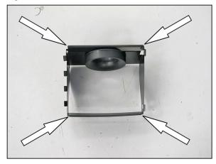
8. Install the two sections of edge trim onto the heat shield as shown. Use the provided super glue to secure the edge trim.
