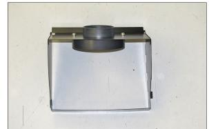
6. Install the filter adapter into the K&N $^{\!0}$  heat shield and secure with provided hardware.
