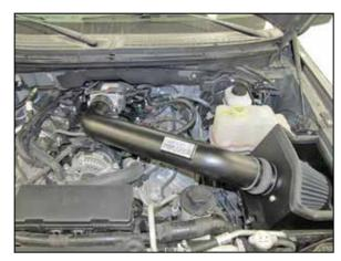
22. Install the K&N® intake tube into the hump hose at the filter adapter and then into the hose at the throttle body, adjust the tube for proper fit and then secure with the provided hose clamps.
