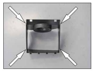
13. Install the cut sections of edge trim onto the bottom of the heat shield as shown.
