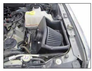
17. Set the heat shield assembly onto the lower air box and secure with the two remaining air box clips.
