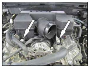
6. Remove the two bolts that secure the intake
