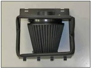
15. Install the K&N<sup>®</sup> air filter onto the adapter and secure with the provided hose clamp.
