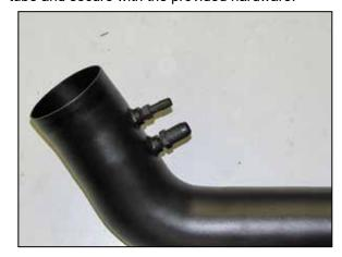
21. Install the two provided NPT vent fittings into the  $K\&N^{\circledcirc}$  intake tube as shown.
