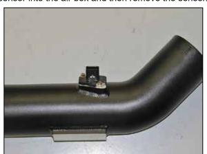
20. Install the mass air sensor into the K&N $^{\rm @}$  intake tube and secure with the provided hardware.
