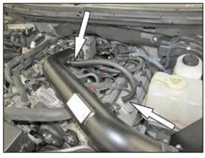
24. Install the provided crank case vent hose onto the valve cover port and then onto the fitting installed into the K&N® intake tube.
