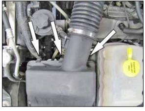
4. Release the three upper air box retaining clips.
