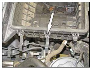
16. Remove the center upper air box retaining clip.
