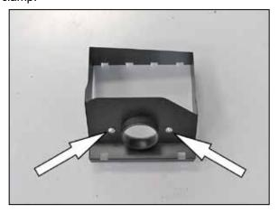
11. Install the filter adapter into the K&N® heat shield and secure with the provided hardware.
