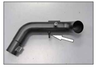
16. Install the provided 3/8" NPT hose fitting into the K&N® intake tube as shown.
