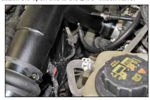
22. Reconnect the mass air sensor electrical connection.
