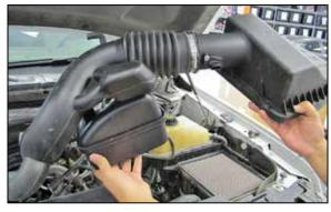
6. Release the three clips securing the upper air box housing to the lower housing and then remove the intake tube/upper air filter housing and air filter from the vehicle.
