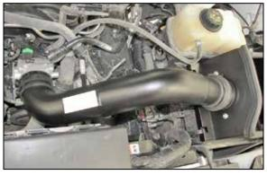
19. Install the intake tube assembly into the silicone hose at the filter adapter and then into the silicone hose on the throttle body and secure with the provided hose clamps.
