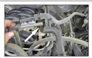
4. Disconnect the EVAP hose from the check valve as shown.
