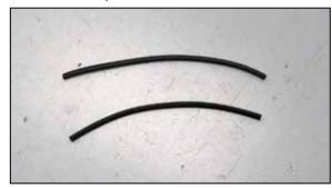
9. Cut the provided edge trim into two 9" sections as shown.
