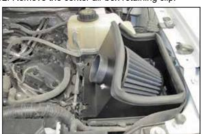
13. Install the heat shield/filter assembly onto the lower air box and secure with the factory air box retaining clips.
