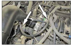
21. Install the provided EVAP vent hose onto the 3/8" fitting installed in the intake tube and then attach the open end to the EVAP check valve.
