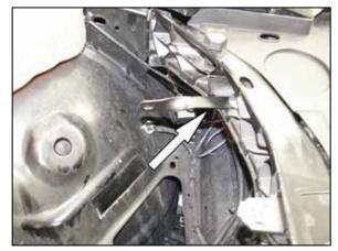
9. Install the heat shield mounting bracket (070772) onto the core support using the provided hardware. NOTE: On vehicles equipped the HID headlights, it will be necessary to install the bolt from bottom up.
