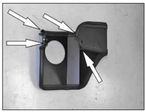
11. Install the two pieces of edge trim onto the heat shield as shown.
