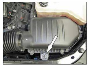
7. Remove the bolt which secures the air filter housing to the core support and then remove the complete air filter system from the vehicle.
