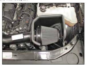
23. Install the filter assembly onto the K&N<sup>®</sup> intake tube and secure with the provided hose clamp.
