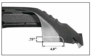
24. Reinstall the engine cover. NOTE: On some models it may be necessary to trim the engine cover for proper fitment as shown.
