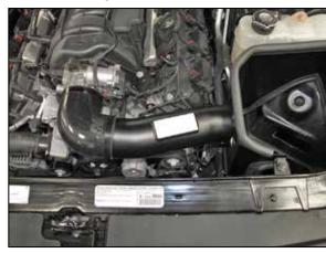
18. Install the K&N® intake tube into the silicone hose and align with the mounting bracket installed earlier. Secure with the provided hardware and hose clamp.
