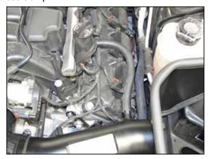
19. Install the provided crank case vent hose onto the fitting on the engine and then connect the open end to the vent on the K&N® intake tube,
