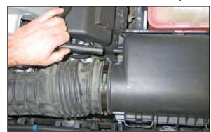
6. On models equipped with a 6.4L, disconnect the crank case vent from the air filter housing as shown.
