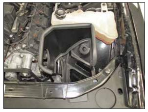
12. Install the heat shield into the vehicle and secure with the provided hardware.
