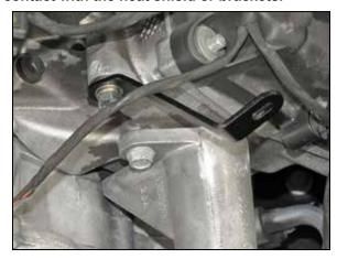
13. Install the tube mounting bracket (010088) onto the cylinder head as shown. Be sure to place the provided spacer between the bracket and cylinder heads.
