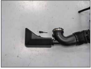
15. Remove the factory inlet air temperature sensor from the factory intake tube.
