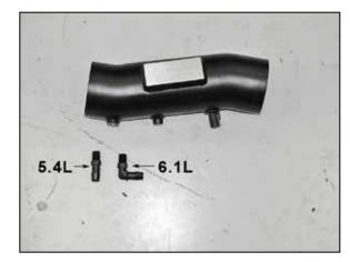
17. Install the appropriate 1/4npt fitting into the K&N® intake tube. The straight fitting is for 5.7L engines and the  $90^{\circ}$  fitting is for 6.0L.
