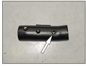
16. Using the provided grommet, Install the inlet air temperature sensor into the K&N® intake tube,
