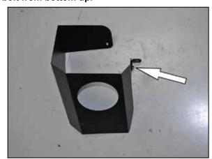
10. Install the heat shield mounting bracket (070066) onto the heat shield as shown using the provided hardware.
