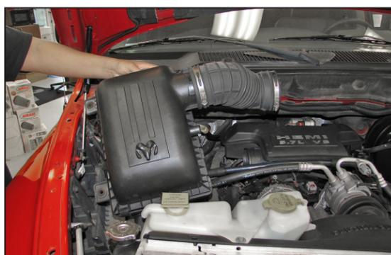
4. Lift up and remove the air filter housing and intake tube from the vehicle.
