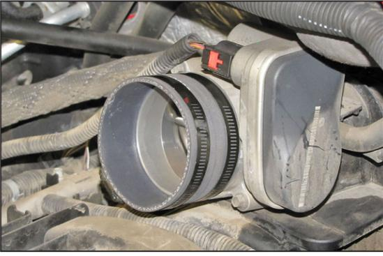
25. Install the provided coupling hose (08698) onto the throttle body and secure with the provided hose clamp.
