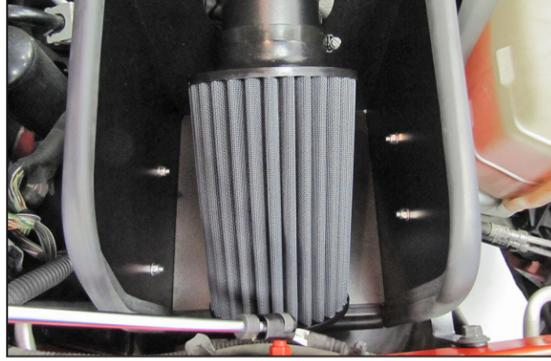
29. Install the air filter and secure with the provided hose clamp.
