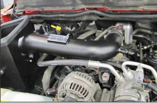
26. Install the intake tube into the heat shield and coupling hose at the throttle body then secure the tube with the hose clamp and hardware,
