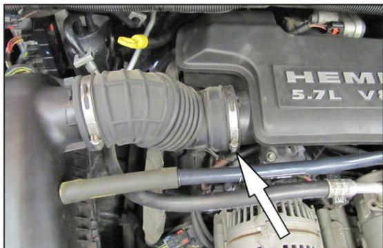
2. Loosen the hose clamp securing the factory intake tube to the intake plenum.
