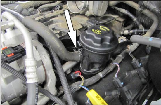
8. Release the spring clamp and then disconnect the crank case vent hose from the breather port.
