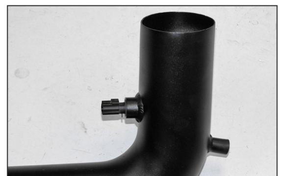
24. Install the inlet air temperature sensor into the silicone hose installed in step #21.
