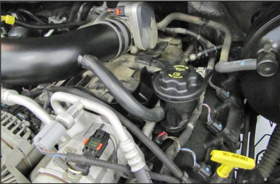
27. Install the provided crank case vent hose onto the valve cover port and then connect the open end to the intake tube.
