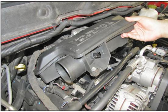
7. Remove the intake plenum and throttle body seal from the vehicle.
