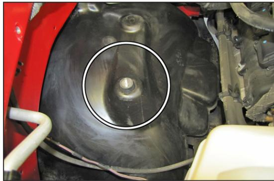
15. Install one of the provided rubber mounted studs onto the inner fender and secure with the provided hardware.
