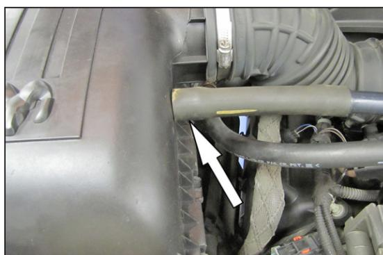
3. Disconnect the crank case vent hose from the air filter housing.
