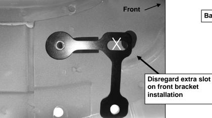
(Fig 3) Front Bracket Spacer on driver side
