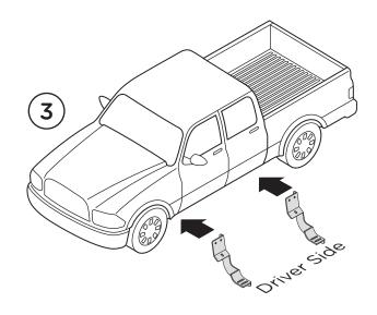
**4.** Align the Front and Rear Driver's Side Brackets with existing bolt and the existing
