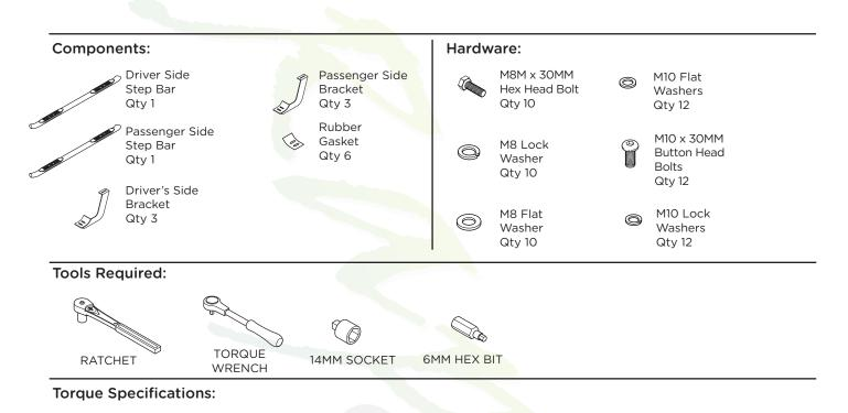
For Rocker Panel Mount Installations M8 through M12 bolts and nuts are set to 15-20 ft lbs.
