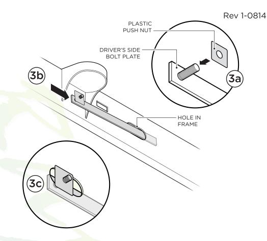
**4.** Align the Driver's Side Front Bracket with the Driver's Side Bolt Plate and secure using one (1) M12 Flat Washer, one (1) M12 Lock Washer and one (1) M12 Hex Head Nut. Hand tighten all hardware.
