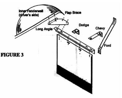
STEP 7: Drill four 1/4" holes into the top of the flap and attach it to the long angle bracket. SEE FIGURE 3
