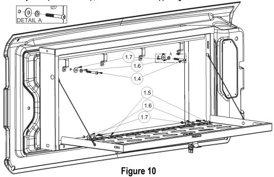
14. Tighten mounting hardware to 8 ft-lbs(10 N-m).
