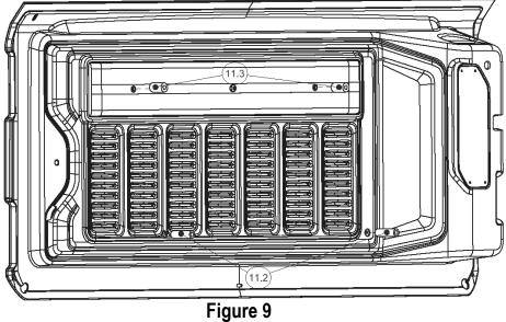
13. While holding the #365 Storage Box in place, insert the mounting hardware through the mounting holes of the #365 Storage Box in the sequence shown in Figure 10. #1.3 Screws (2") are used in the upper mounting holes, and #1.5 Screws (2 3/8") in the lower holes. NOTE: This step is most easily accomplished with help, or another means of supporting the lockbox at the correct elevation.
