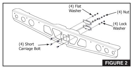
Orientate flat surface of clamp assembly with backside of frame so nuts on long bolts face down. Attach clamps to frame with (4) short carriage bolts, flat washers, lock washers so nuts face vehicle. Leave all bolts loose for now.
