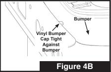
Position support flange on bumper step (Figure 4A) and push frame tight against bumper until both vinyl bumper caps are "tight" against vehicle bumper (Figure 4B).
