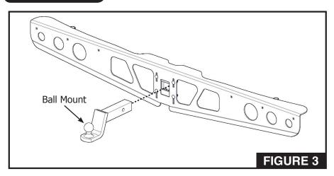
Slide ball mount through frame and clamps. Lift assembly up and insert ball mount into receiver tube. Secure with pin and clip.
