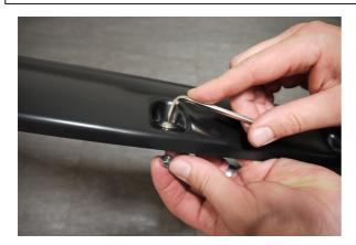
**STEP 1:** Attach the 11 bolts and nuts to each Fender Flare using a 3/16" Allen key and a 1/2" wrench/socket. wrench/socket. (wrench /socket and Allen key not supplied). Ensure inside of Fender Flares where the rubber seal is attached is clean, using the alcohol wipes provided. Wipe away any residue with a dry clean cloth.
