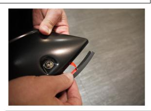
**STEP 2:** Attach the included rubber seal to the Fender Flares. Peel back 2" of the adhesive backing and position on the Fender Flare. Attach the seal to the Fender Flare, peeling back a few inches at a time. Ensure pressure is used to secure rubber seal to Fender Flare edge. Attach rubber seal along all areas the Fender Flare will make contact with the vehicle body. Trim excess rubber seal.
