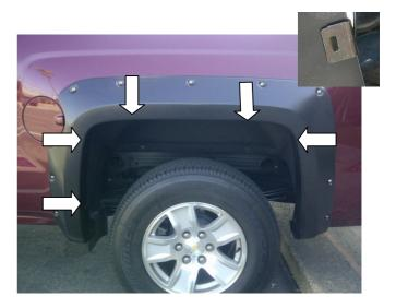
**STEP 6:** To secure the Fender Flare to the body, apply upward tension on Fender Flare to the vehicle fender when installing the black metal clips. Slide the clips over the Fender Flare and the inner wheel arch lip in the five locations shown. Position the clip so that the barb in the clip locates in the slot of the Fender Flare.
