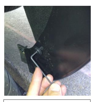
**STEP 8:** Using #15 Torx head screwdriver reinstall the upper screw from the rear factory mudguard through the slot in the Fender Flare.
