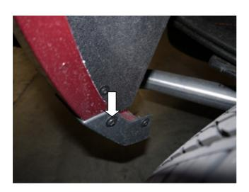
**STEP 5:** Using #15 Torx head screwdriver remove upper screw from the rear factory mudguard. Maintain screws for re-install.
