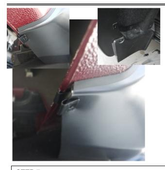
**STEP 7:** Slide the top edge of rear front mudguard cut out behind the factory mudguard. Install the E shape clip so that the clip slides over the inner sheet metal lip and is in line with the slot in the underside of Fender Flare. To secure the clip to Fender Flare apply inward tension on Fender Flare to the vehicle fender when installing the E clip, position the clip so that the barb in the clip locates in the slot of the Fender Flare.
