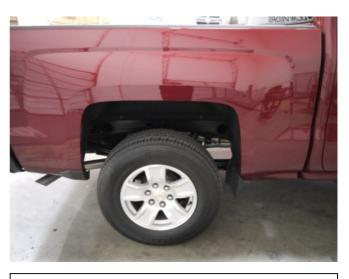
**STEP 4:** Clean the body areas where the Fender Flares will make contact. Ensure fenders are dry prior to install.
