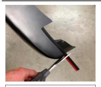
**STEP 3:** Attach rubber seal to the bottom front corner of Fender Flares. Peel back 1" of the adhesive backing and position on the Fender Flare. Attach the seal to the Fender Flare, ensure pressure is used to secure rubber seal to Fender Flare edge. Trim excess rubber seal and discard.
