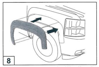
Place the front Fender Flares onto the vehicle and line up the holes on the part with the screw holes on the vehicle.
