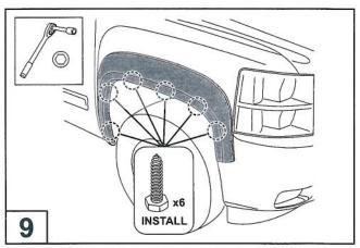
Re-Install the socket head screws into the fender to secure the Fender Flares. Fit the Fender Flares loosely until the Fender Flares are aligned as desired, when satisfied, tighten the screws fully and ensure extrusion is flush neatly against the body.
