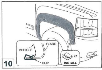
Install 1x wheel arch clip as shown.
