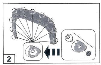
Attach 10 bolts to each Fender Flare using a 3/16" Allen key and a 1/2" wrench/socket.
