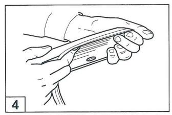
Remove approximately 2" (50mm) of the protective liner from the extrusion. Fit the extrusion to the Fender Flare along the edge that comes in contact with the vehicle's body panel.
