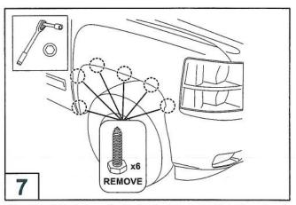
Use the original manufacturer's hardware that is in the wheel arch of the vehicle to fit the Fender Flares. Remove the 6x 7mm socket head screws from the fasteners on the vehicle.
