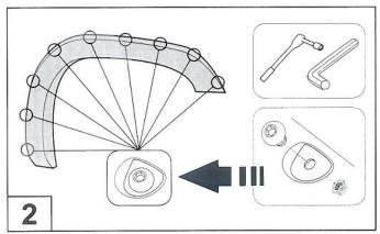
Attach 9 bolts to each Fender Flare using a 3/16" Allen key and a 1/2" wrench/socket. (wrench/socket and Allen key not supplied)
