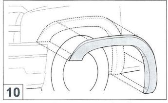
Place the Fender Flare into the position of best fit.
