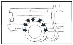
**9.** Remove the previously noted existing screws and retain for re-installation.
