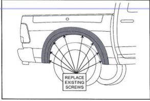
10. Replace Fender Flare on the vehicle into position of best fit. Complete installation by replacing the previously removed screws at position A-H, ensuring the Fender Flare is located firmly and extrusion is neat against the vehicle fender.
