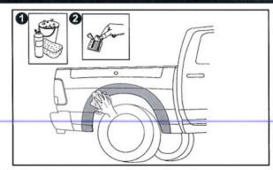
Wash the areas of contact on the vehicle and wipe dry both the vehicle and the Fender Flares with a clean cloth. Ensure inside of Fender Flares where extrusion is attached is clean, using the alcohol wipes provided and wipe away any residue with a dry, clean cloth.
