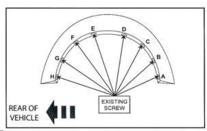
7. Note the correct hardware for positions A-H (Right Fender Flare shown).
