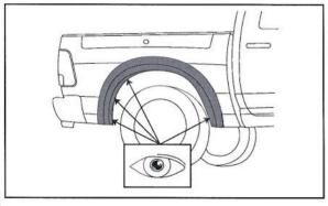
Place the Fender Flare on the vehicle into the position of best fit. Note where the slots in Fender Flare at positions **A-H** align with the existing screws in the vehicle. Remove Fender Flare.
