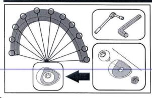
2. Attach 11 bolts to each Fender Flare using a 3/16" Allen key and a 1/2" wrench/socket. (socket wrench and Allen key not supplied)
