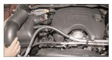
Using a flathead screwdriver, loosen the clamp at air filter box and lift the intake hose out of the way.
