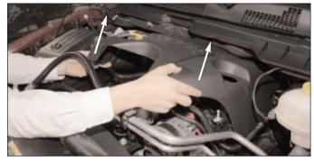
Remove the engine cover by pulling it up.
