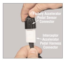
Plug the Interceptor accelerator pedal harness connector into the vehicle's factory accelerator pedal sensor connector. Position the Interceptor Accelerator Controller out of the way of the accelerator. Installation is now complete.
