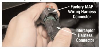
Plug the Interceptor harness connector into the factory MAP wiring harness connector, and push in the locking clip. Reinstall the engine beauty cover then the intake hose removed in the previous steps. **DO NOT reconnect the air intake sensor as it will be reconnected in the next section of the Interceptor installation.**
