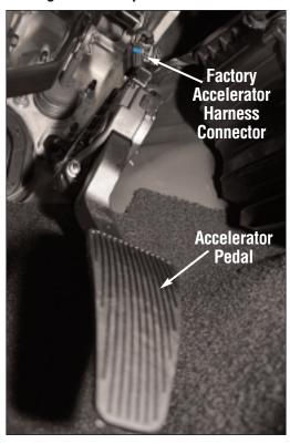
Using a flashlight, locate the factory accelerator harness connector under the driver's dashboard and above the accelerator pedal. Disconnect the factory harness from the accelerator pedal sensor.
