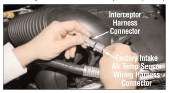
Plug the Interceptor harness connector into the factory intake air temp sensor wiring harness connector.
