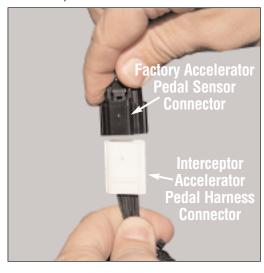
Plug the Interceptor accelerator pedal harness connector into the vehicle's factory accelerator pedal sensor connector. Position the Interceptor Accelerator Controller out of the way of the accelerator. Reinstall the two (2) connectors to the module behind the dash panel and the metal plate removed from Step 2, then reinstall the dash panel removed in Step 1. Installation is now complete.
