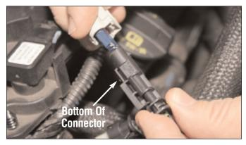
Plug the Interceptor harness connector into the factory 3-Pin sensor wiring harness connector. *NOTE: The correct orientation of the connector is shown above.*
