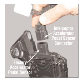
Plug the Interceptor accelerator pedal sensor connector into the factory accelerator pedal sensor.
