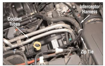
Route the Interceptor harness toward the air inlet box, and then back to the 4-Pin cam sensor. *Use the provided zip ties to route the Interceptor harness away from coolant tubes.*
