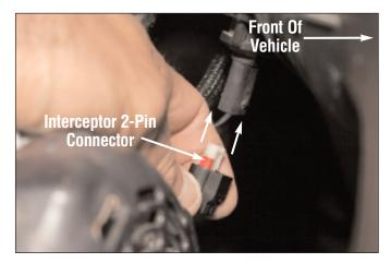
Route the Interceptor harness under the air intake, and plug the Interceptor 2-Pin connector into the vehicle intake air temp sensor. *NOTE: The correct orientation of the connector is shown above.*
