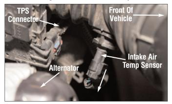
Disconnect the factory connector from the 2-Pin (intake air temp) sensor.
