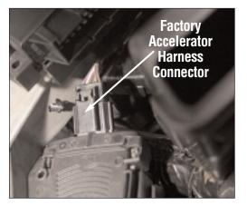
Disconnect the factory harness from the acceleratoe pedal sensor. Using a flashlight, you should see the accelerator pedal connector just behind the module which was unplugged in t he previous step. This picture is taken from the pedal area, looking up toward the windshield.
