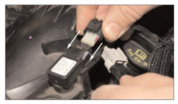
Plug the Interceptor 3-Pin connector into the vehicle MAP sensor.
