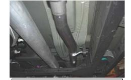
3. Install muffler assembly Item # B onto the head pipe 6". You may need to use a jack stand to support the muffler while installing the tailpipe. Use Item# E to clamp the muffler assembly to the head pipe. Loosely tighten down.
