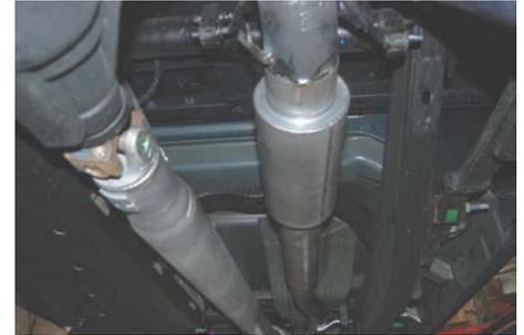
4. Install over axle pipe Item # C into the muffler outlet. Slip the hangers into the rubber grommets and keep tailpipe loose.
