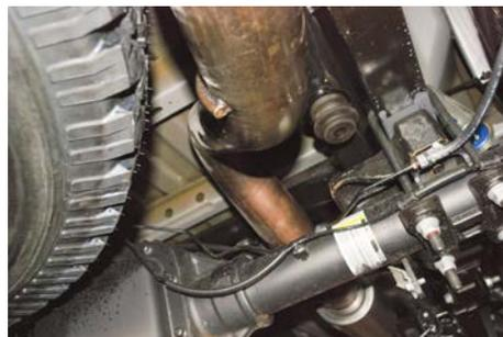
6. With proper clearance from spare tire install the exhaust tip onto the tailpipe. The system was designed to have the tip 1" below the quarter panel of the vehicle. With the tip in your desired position begin to tighten down all clamp connections from the front head pipe back.
