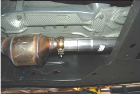
2. Install Head pipe Item # A onto the factory flange. You will re use the factory clamp at this connection. Loosely tighten down the clamp.
