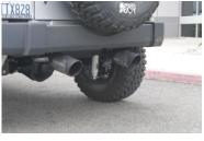
4. Install stainless steel tips. Clamp down. When you have everything in place, firmly tighten all bolts and clamps down securely. Use stainless steel cleaner and a Scotch Brite pad weekly to prevent tip from discoloration. Inspect all fasteners after 25-50 miles of operation and re-tighten as necessary.
