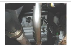
4. Install Over axle pipe Item # A onto the factory head pipe. Use clamp Item D to secure but do not tighten.
