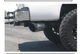
7. With proper clearance from spare tire and the tip in your desired position begin to tighten down all clamp connections from the front head pipe back to the tip.
