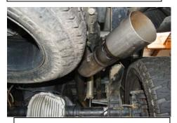
**5.** Install the exit pipe Item #C Be sure there is clearance from the spare tire and shock. You may need to adjust the pipes for a proper 1.50" of clearance.
