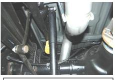
4. Install Over axle pipe Item # B onto the head pipe. Use clamp Item E to secure but do not tighten.
