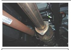
2. Be sure to not damage the gasket and bolts they will be re used for the exhaust install.
