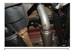
5. Install the over axle pipe. With everything loose you may need to adjust the system for proper clearance of shocks, brake lines, ect.
