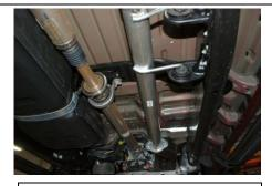
3. With the head pipe and hangers in position install the muffler assembly Item # B. You will use the Clamp Item # E to secure to the head pipe. Do not tighten keep loose.
