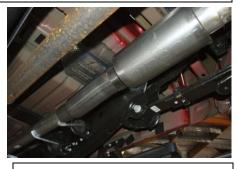
4.Use a jack stand to support the muffler assembly until you have installed the over axle pipe Item # C
