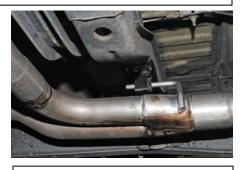
4. Install the Resonator Item #B onto the head pipe Item # A. The inlet of the resonator will have the louvers opening towards the front of the vehicle. Install extension pipe Item # J onto the resonator. Loosely tighten down.
