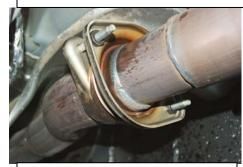
2. Install muffler assembly Item # A into the factory head pipe. Use the clamp Item # E at this connection. Install hanger into rubber grommet and loosely tighten down the clamp.
