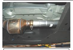
2. Install Head pipe adapter Item # G onto the factory flange. You will re use the factory clamp at this connection. Loosely tighten down the clamp. Install headpipe Item # A onto the adapter. Loosely tighten down.
