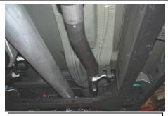
3. Install muffler assembly Item # B onto the head pipe. You may need to use a jack stand to support the muffler while installing the tailpipe. Use Item# E to clamp the muffler assembly to the head pipe. Loosely tighten down.
