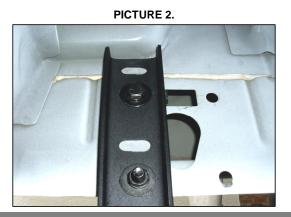
6.- Mount the side bar to the brackets and attach with: 5/16 x 1 1/4" hex head bolt, 3/8" flat washer, 5/16" lock washer. By each bracket. Leave loose. **SEE ILLUSTRATION 3 & 4.**
