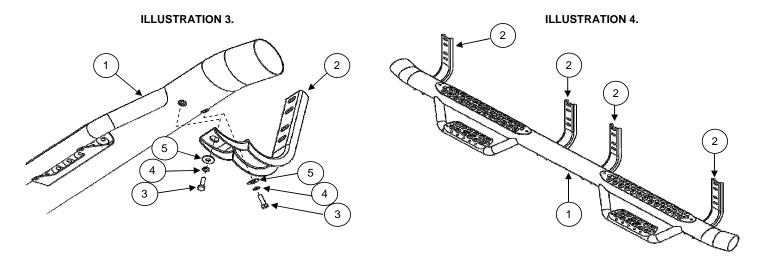
7.- Make any final adjustments to the alignment of the bracket and tighten all bolts.
