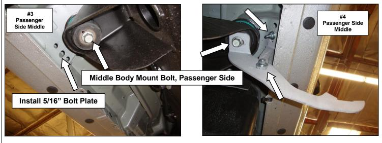
**Step-5** Remove the passenger side rear body mount bolt. Keep all existing washer and bushing in place, and attach the passenger side rear bracket to the vehicle using the factory body mount bolt and supplied 1/2" flat washer, (Photo 5 & 6). Leave the body mount bolt loose for final adjustment.
