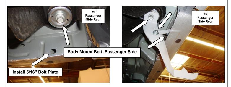
Step-7 Attach the passenger side step to each of the brackets using (2) 5/16" x 1" hex bolts, (2) 5/16" lock washers and (2) 5/16" flat washers, (Photo 7).
