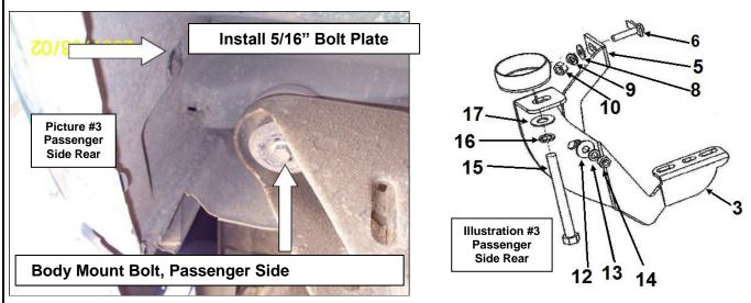
**Step-7** Attach the passenger side step to each of the brackets using (2) 5/16" x 1" square head bolts, (2) 5/16" flat washers and (2) 5/16" lock washers as shown. **Illustration #3 & #5**
