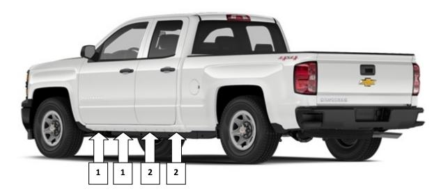
Before beginning the installation, please read all directions carefully and verify that all necessary hardware is accounted for. If any parts are missing, stop the installation and contact your distributor immediately. This installation uses 2 front and 2 rear brackets per side.
