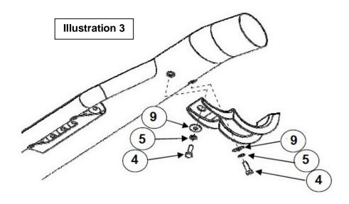
**Step-6** Align the side bar with the vehicle and tighten all side bar and bracket nuts and bolts. Repeat the installation steps to install the passenger side brackets and side bar. Remember to check and retighten all nuts and bolts periodically.
