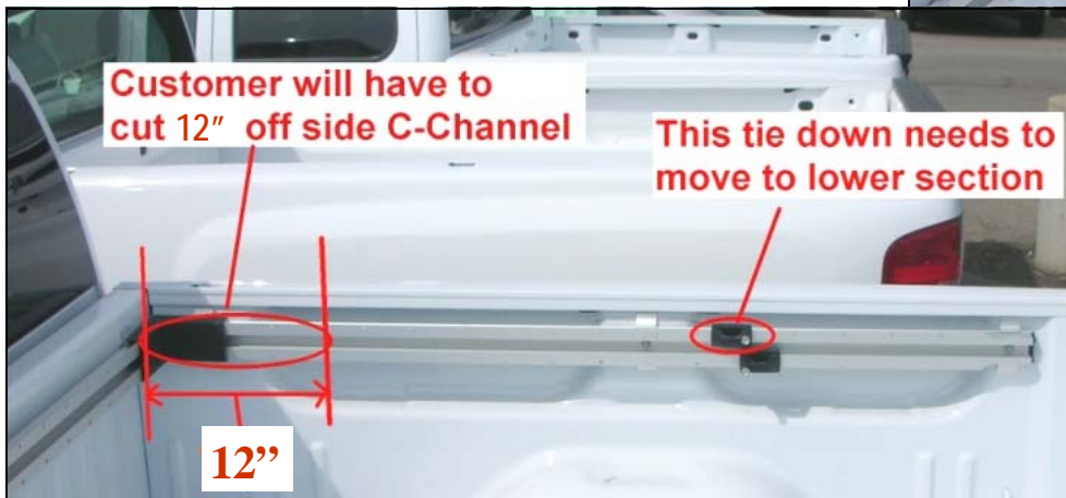
PHOTO 2 — Option 1 for side rail modification.
