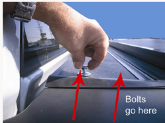
Step 5. Push provided bolts through holes and plate and tighten under cover, using provided nuts and washers.
