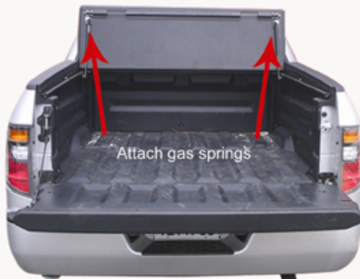
Step 6. Attach provided shocks to connectors on cover and rails. Attach drain tubes.
