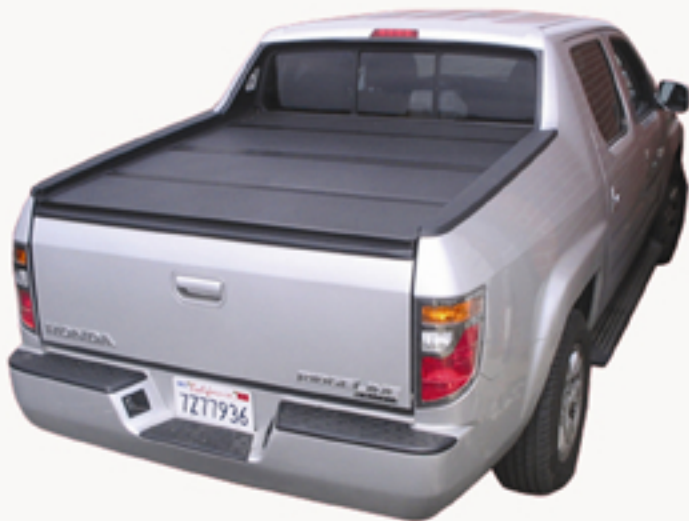
Step 3. position cover squarely on rails. Make sure the cover sits against cab and on top of tailgate.
