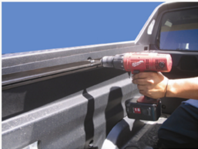
Step 2. Attach rails to side wall. Make sure rails are positioned hard up against cab wall. Use smaller diameter screws in middle and larger at front.
