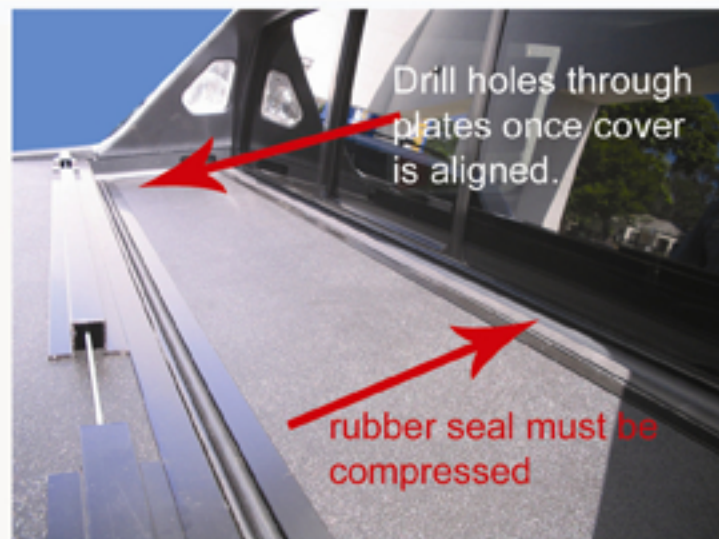
Step 4. Push Cover HARD up against cab. Rubber seal should be compressed slightly. Drill a hole with an 11/32" bit through the plates that extend out of your Bakflip rails. (2 on each side)
