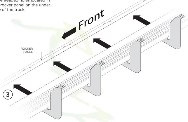
**4.** Fasten Driver's Side Brackets to the Rocker Panel using two (2) M8 x 30MM Hex Head Bolts, two (2) M8 Lock Washers, and two (2) M8 Flat Washers per bracket.
