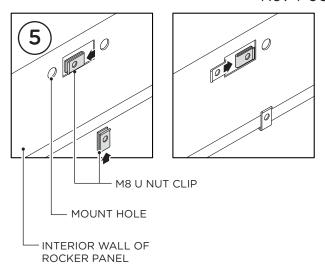
**6.** For the Center and Rear Brackets, on the vertical wall of each rocker panel, install the three (3) U Nut Clips as shown.
