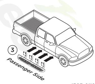
1 1303-0119 **5.** For the Front Brackets on the vertical wall of each rocker panel, install the three (3) U-Nuts as shown. Two (2) U Nut Clips are to be installed covering the two (2) mount holes and one (1) U Nut Clip is to be installed on the bottom of the body panel. Install these U Nut Clips so that the threads are to the inside of the rocker panel. Be careful not to drop the U Nut Clip inside of the rocker panel.
