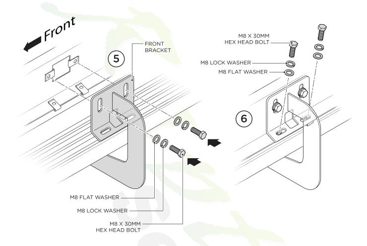
Repeat these steps for driver side installation. When all hardware is in place, everything must be tightened. See Page 1 for Torque Specifications.
